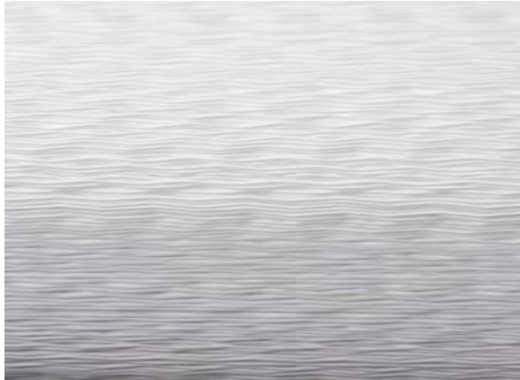
a) undulated fibers that promote even dialysate flow
